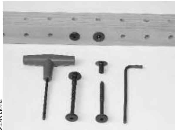
1.9: Tools and fasteners for wooden grid beam. The T-handled Allen wrench at left is easy to use; the L-shaped wrench at right is better for tight spaces.
