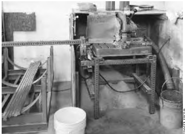
1.17: Steel-framed stand for a chop saw that cuts bronze bar. Built in 1980 as part of an industrial assembly line, it is still in use.
