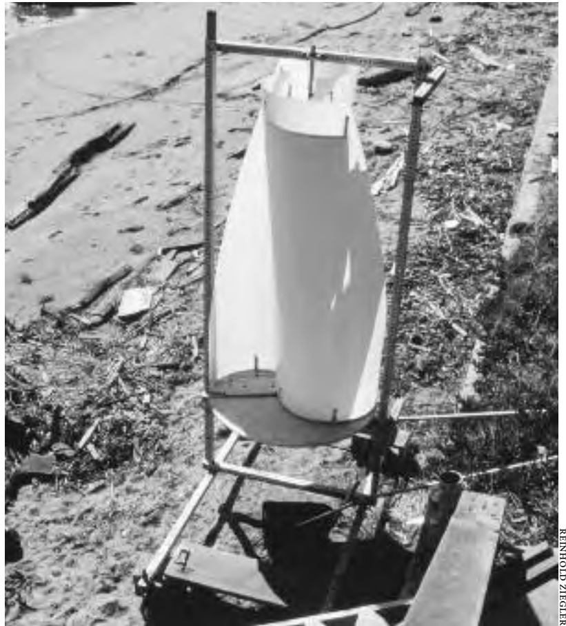
1.4: Steel-framed HELIOS helical rotor. Designed by Reinhold Ziegler and built by students in 1985, it uses Filon fiberglass rotors to pump water.
