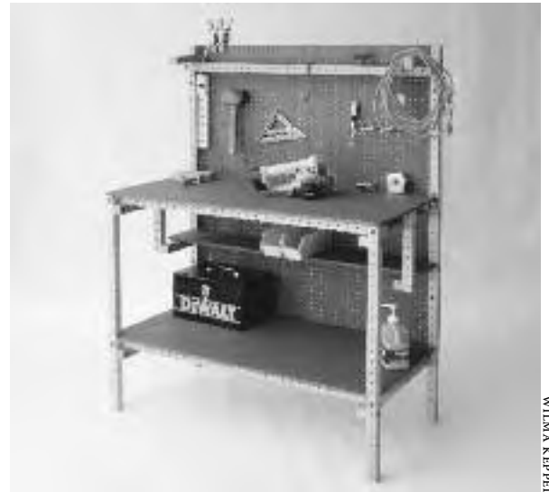
1.11: The Twelve-Minute Workbench. The small shelf can also go on top.
