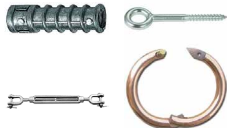
1.7. Equipment needed for the center pipe method: leaded expansion shields to insert into slab ( upper left ); eye bolt to go into the expansion shield ( upper right ); turnbuckle for tensioning the guy wires ( lower left ); opening O-ring to slide up and down the center pole ( lower right ).
