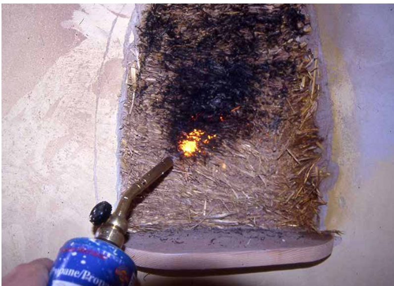
Even with the intense heat application of a blow torch, LSC only smolders.
