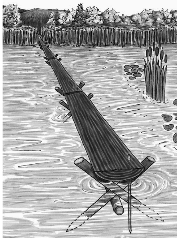
FIGURE 1.4: The Sweet Track was an elevated walkway fashioned using oak planks and coppice-derived stakes that connected hilltop settlements in this seasonally inundated lowland habitat.
